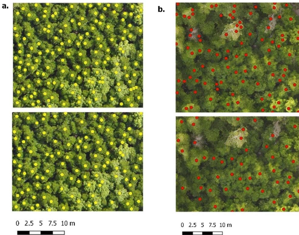
**Fig. 6.** Trees detected in the CHM. Example of the location of the trees detected by the algorithm in the productive zone (a) and in the protective zone (b). The upper image correspond to the set of parameters using all the trees measured in the field, and the bottom image correspond to the parameters using only the trees that form the upper canopy (see Table S2, supplementary material).
