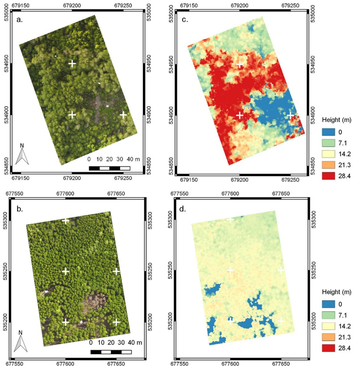
Fig. 5. UAV data derived products. Orthomosaic images of the protective zone (a) and the productive zone (b). CHM generated for the protective zone (c), and the productive zone (d).
